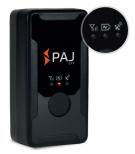
Wait for the end of the charging process. The unit is fully charged when the red LED goes out, see "1.10 Meaning of the LED lights" of this manual.
